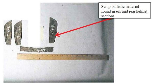
Figure 10: Scrap ballistic material inserted into ear and back sections.
