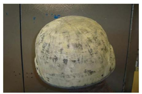
Figure 5: Damaged ACH after paint removal.
