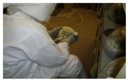
Figure 3: Inmate using power sander to remove paint.
