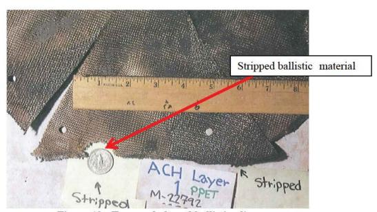
Figure 12: Torn and altered ballistic plies.
