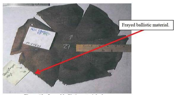
Figure 13: Jagged ballistic material edges.
